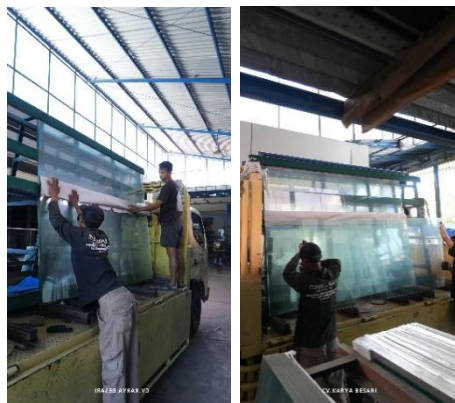
Figure 1. Loading of Large Glass Sheets onto Transport Vehicles (Source: CV Karya Besari internal documentation, 2026)
