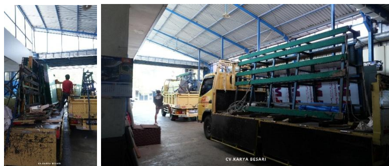
Figure 2. How to use special support racks (A-frames) to protect products (Source: Internal CV Karya Besari documentation, 2026)
